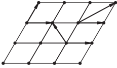
Fig. 1.3: Example of a two-dimensional Bravais lattices without a basis (the lattice nodes are atoms).
